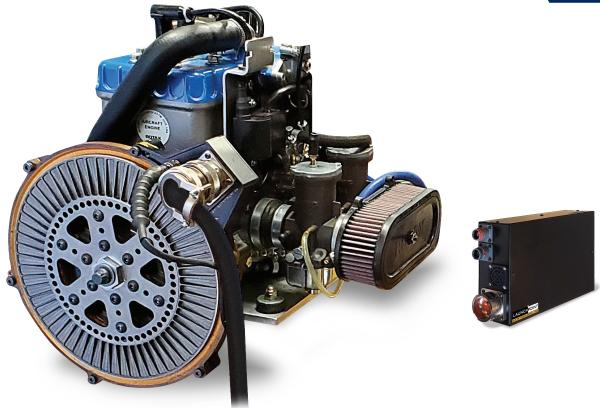
The LaunchPoint® HPS400 Genset is a 40 kW, highly efficient, high specific power generator and hybrid electric power/engine controller system that utilizes patented electric machine and genset technology to enable extended range flight.
