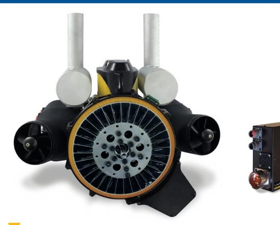
The LaunchPoint HPS055 GenSet is a 5.5 kW, highly efficient, high specific power generator and hybrid electric power/engine controller system that utilizes patented electric machine and GenSet technology to enable extended range flight.
