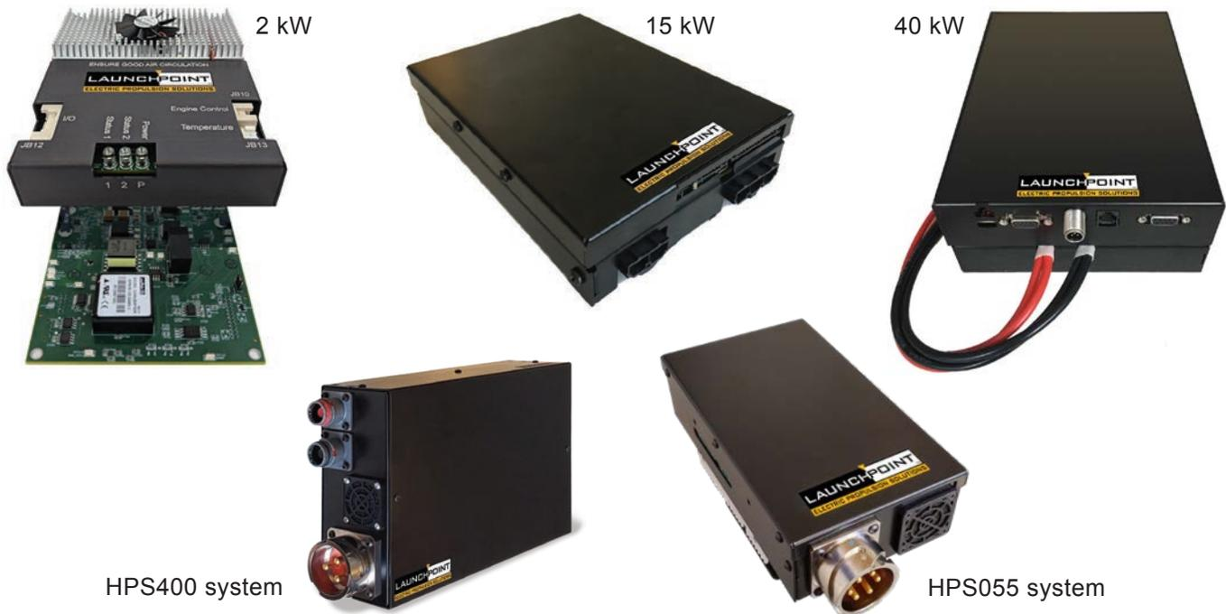
**LaunchPoint's Controllers** are advanced electric motor drives, generator controllers, and hybrid electric power system management units that are designed for all electric and hybrid electric propulsion applications.
